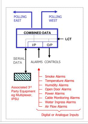
The SP-15 Remote Terminal Unit (RTU) addresses the need for a cost effective solution to integrate third party equipment(s) with proprietary protocols into a common management solution. Additionally a configurable number of control outputs and alarm inputs, including analogues can be accommodated.
